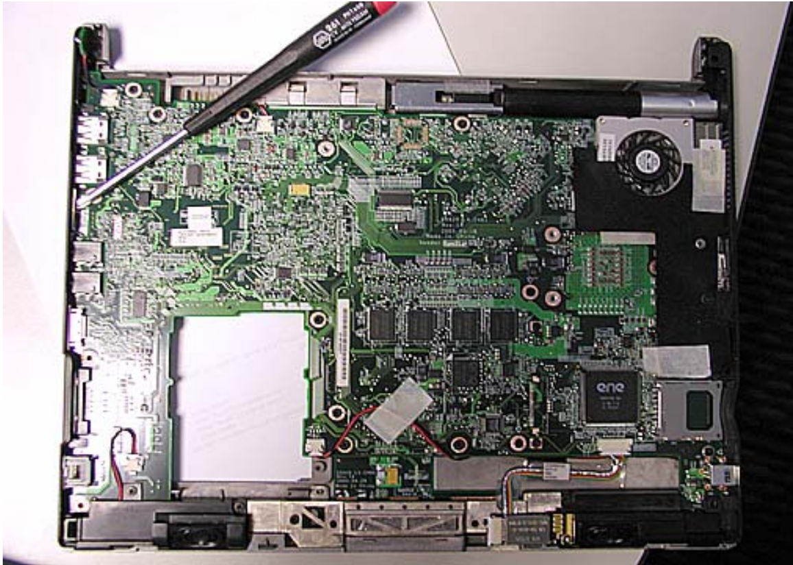
LE1600 Aux Antenna Location 2
