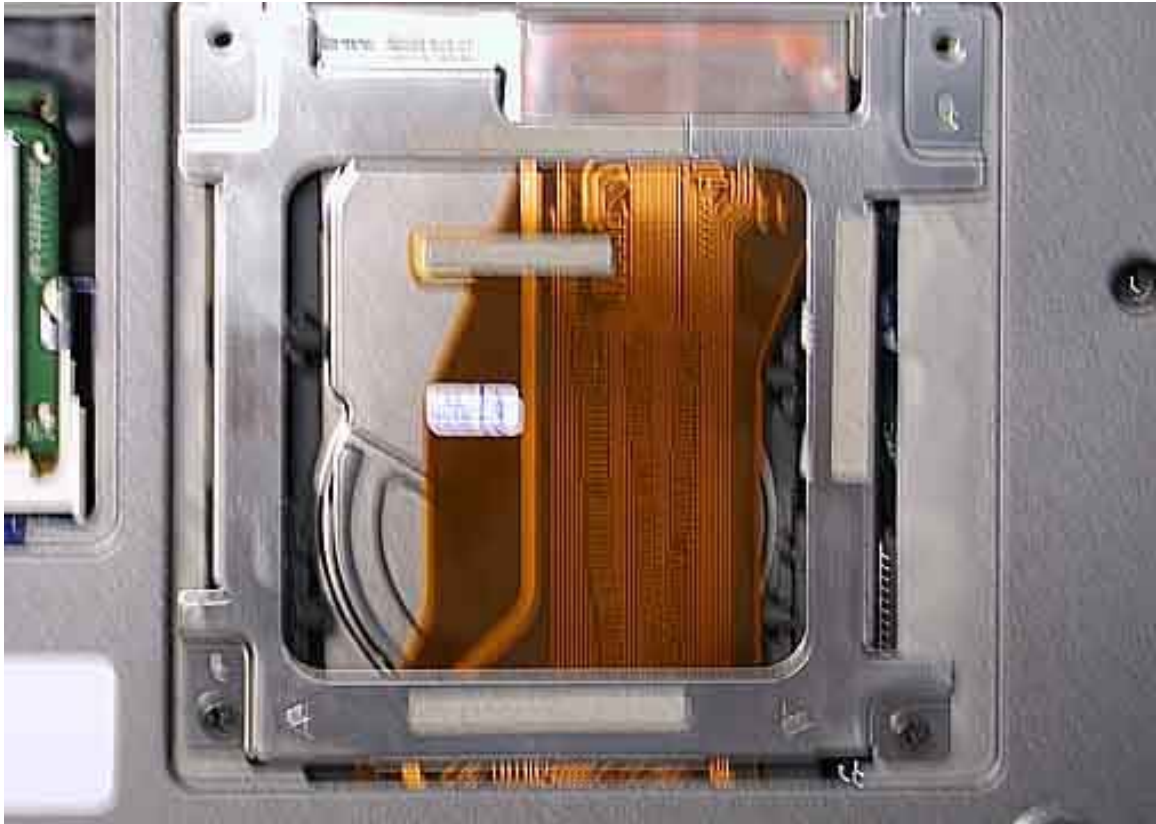
LE1600 HDD Location
