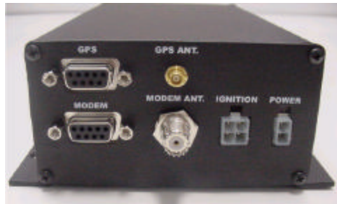
Figure 3 – iR1200 Rear Panel Layout
