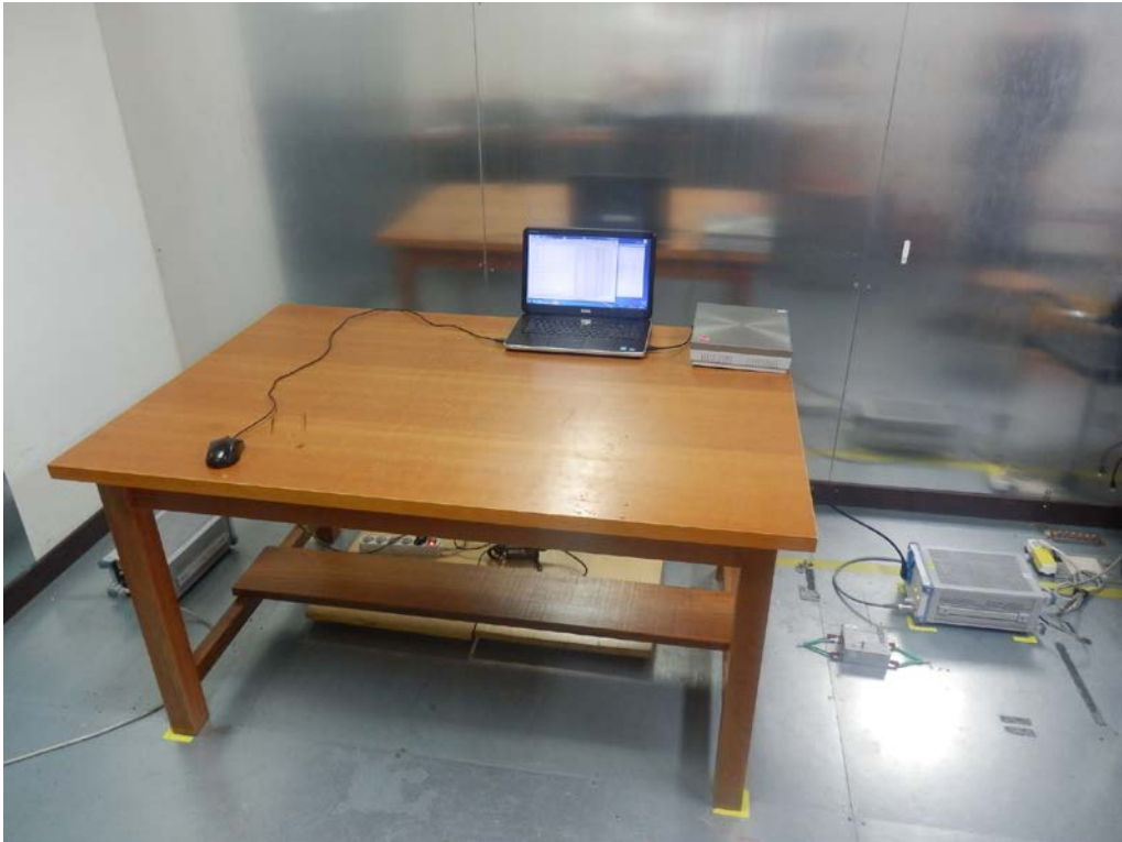
Photograph 3: Test Setup for Conducted Emission
