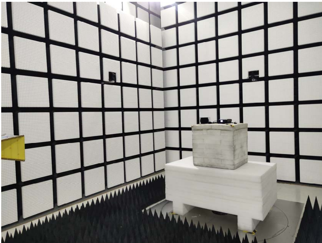
Radiated Emission Above 1GHz View
