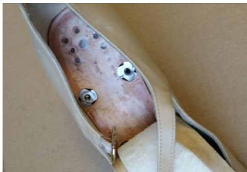
Figure 4 - T-Nuts installed into sole
