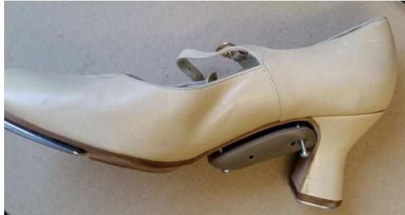
Figure 5 - Transmitter Pod attached to Shoe
