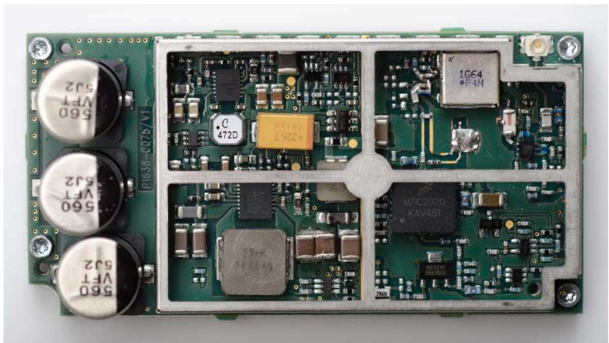
Figure 2 – 9523N rev B/V1 – Top View with screening can lid removed
