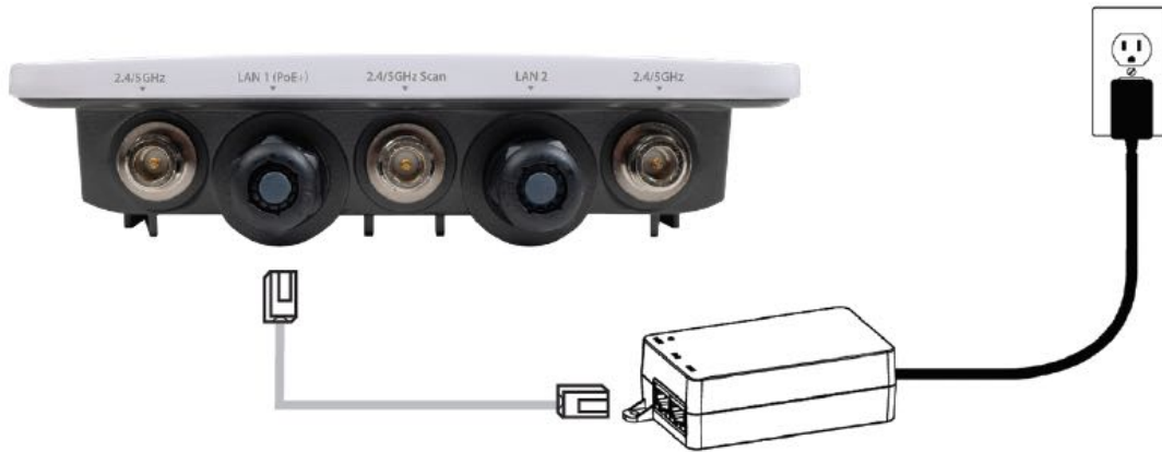
Access Point connected to PoE+ injector
