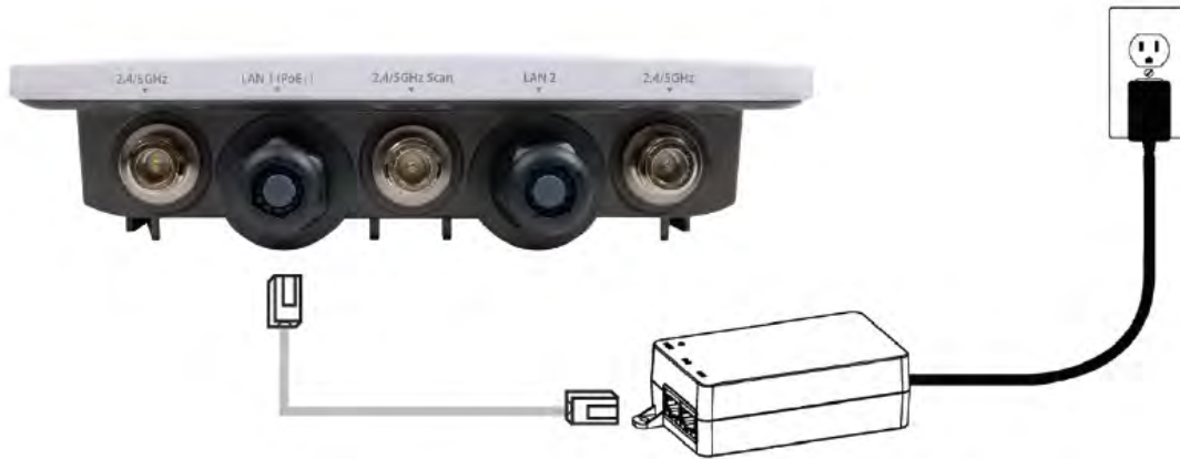
Access Point connected to PoE+ injector
