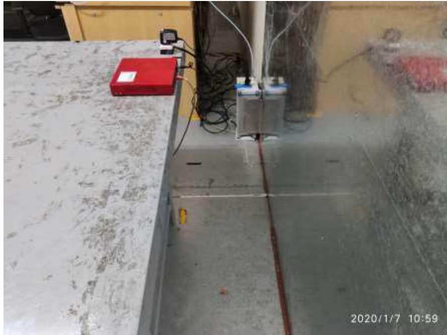
Photograph 7: Set-up for Mains Conducted testing (Back View)
