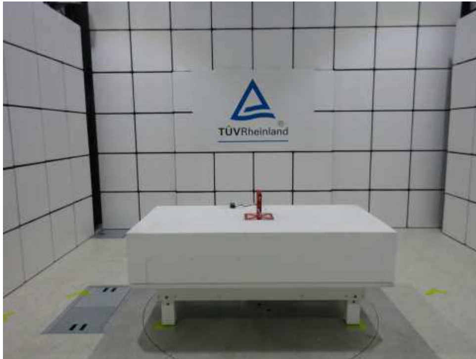
Photograph 1: Set-up for Spurious Emissions (Front View 1)
