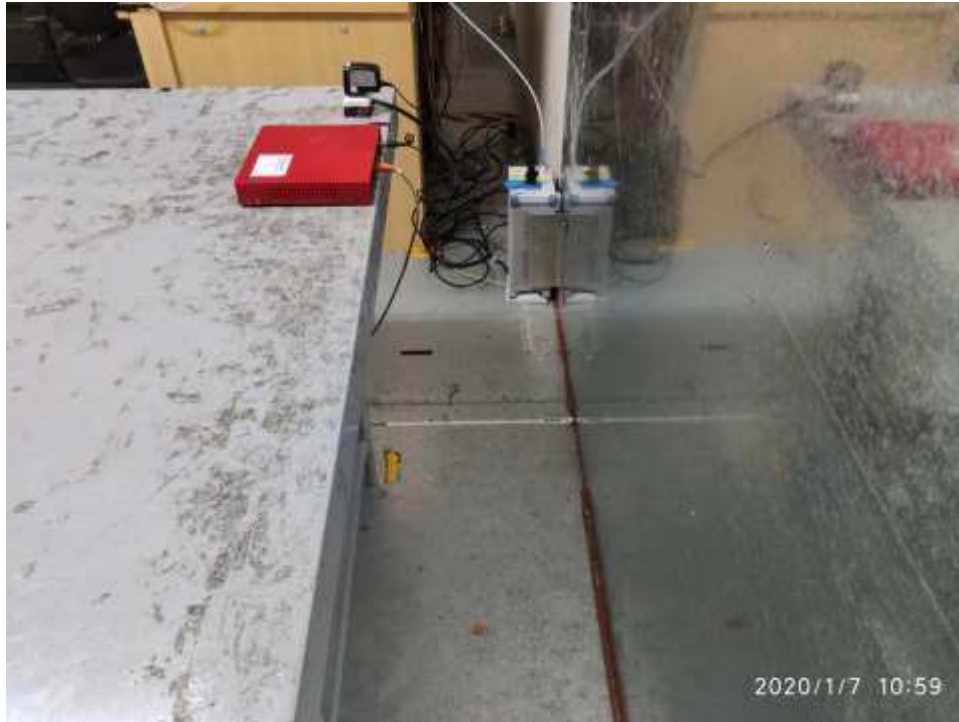
Photograph 7: Set-up for Mains Conducted testing (Back View)
