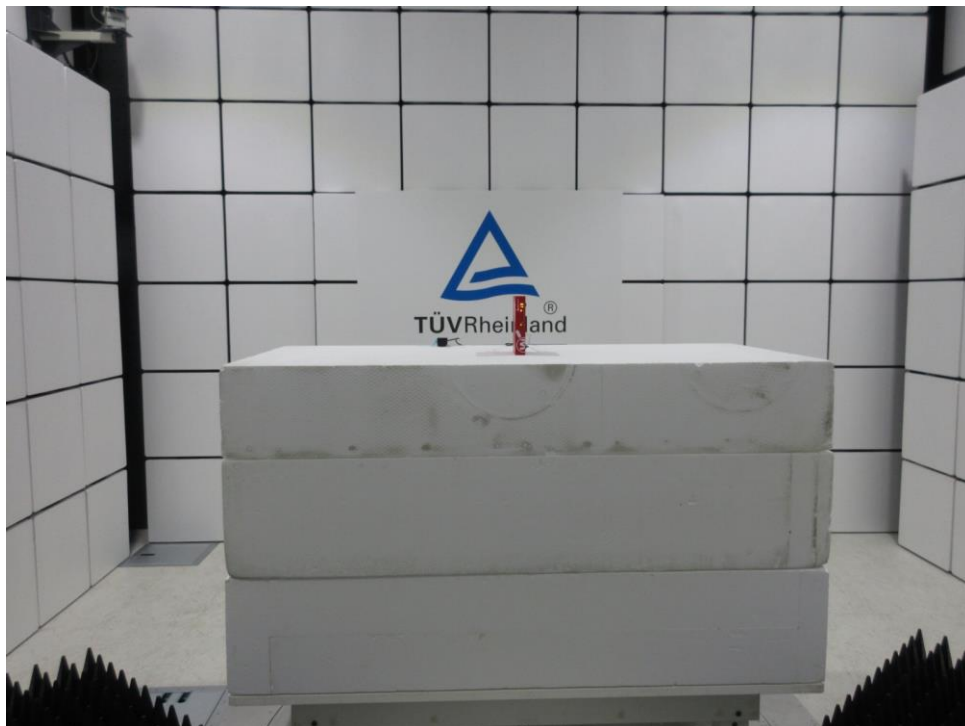
Photograph 2: Set-up for Spurious Emissions (Front View 2)
