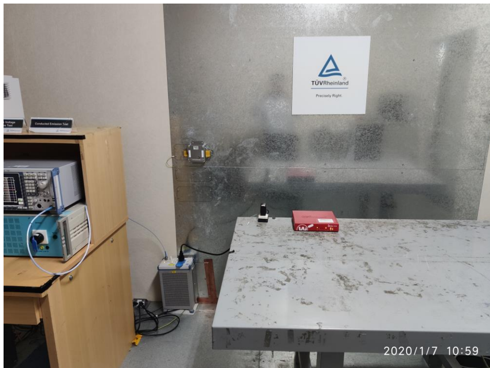
Photograph 6: Set-up for Mains Conducted testing (Front View)
