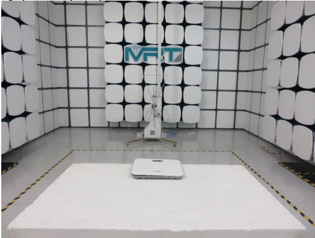
Photograph 2: Set-up for Spurious Emissions below 1GHz
