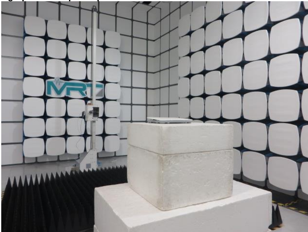
Photograph 3: Set-up for Spurious Emissions above 1GHz
