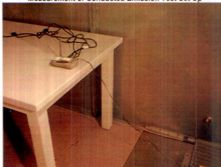
Measurement of Conducted Emission Test Set Up
