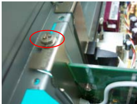
Fig. 3 Secure the card by the screw
