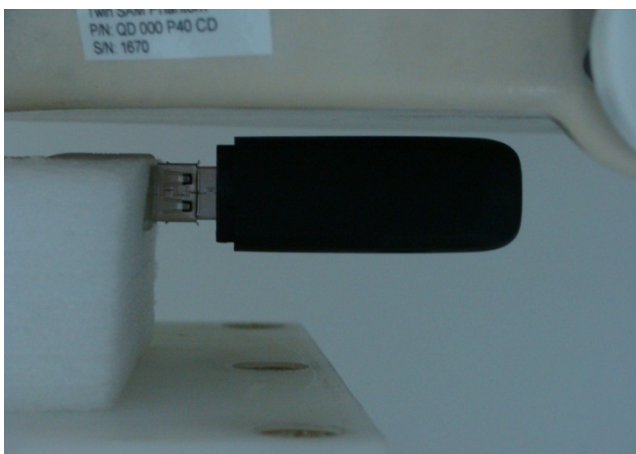
USB Cable Plug-in for USB Configuration 3 Vertical Front with Phantom 0.5 cm Gap
