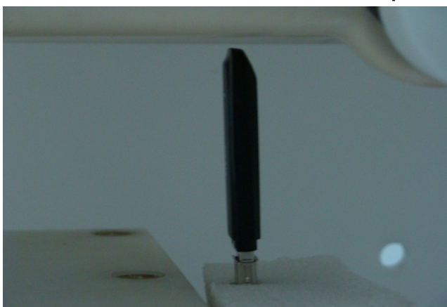
USB Cable Plug-in for USB Configuration 5 Tip Mode with Phantom 0.5 cm Gap
