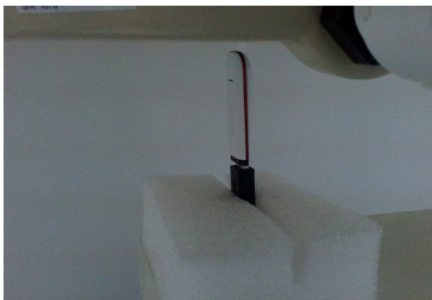
USB Cable Plug-in for USB Configuration 5 (Tip Mode with Phantom 5 mm Gap)
