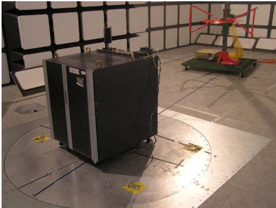
Radiated Emission - Front View (Below 1 GHz)
