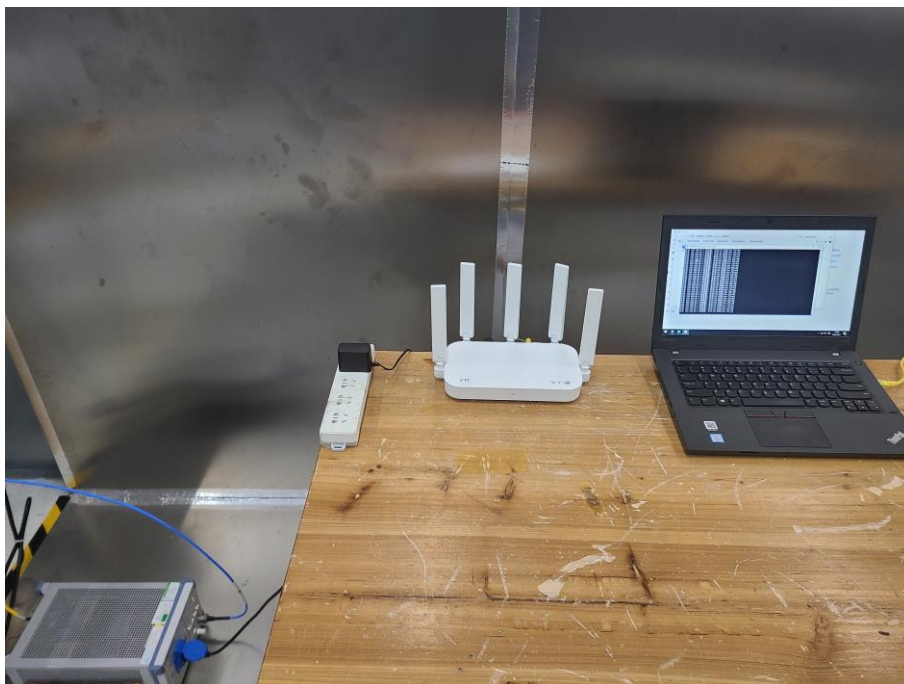
Photograph 3: Set-up for Conducted Emission on AC Mains
