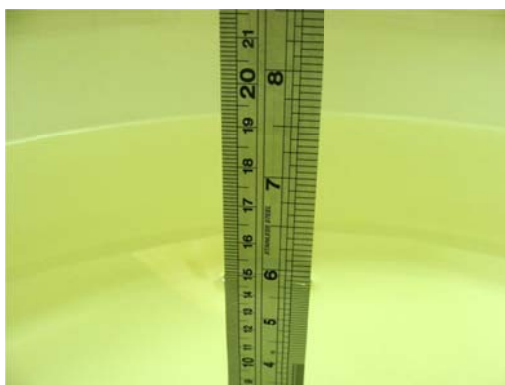
Fig 6.1 Photo of Liquid Height for Body SAR
