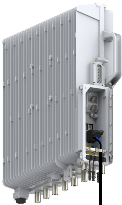
Figure 3-7 Connection of DC Power Input Cable
