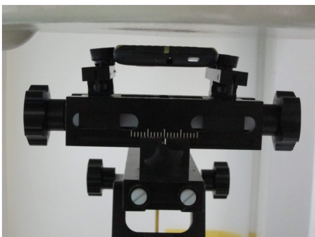
Front Face of DUT with Phantom 1 cm Gap
