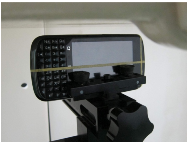
Back Face of DUT with Phantom 1 cm Gap
