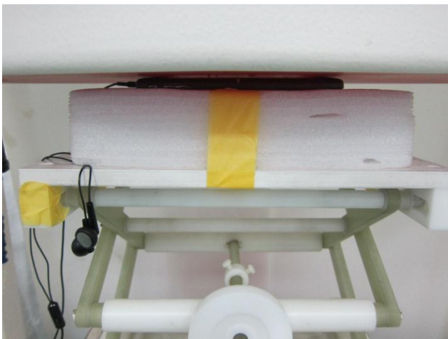
Bottom Face of the EUT with Phantom 0cm Gap
