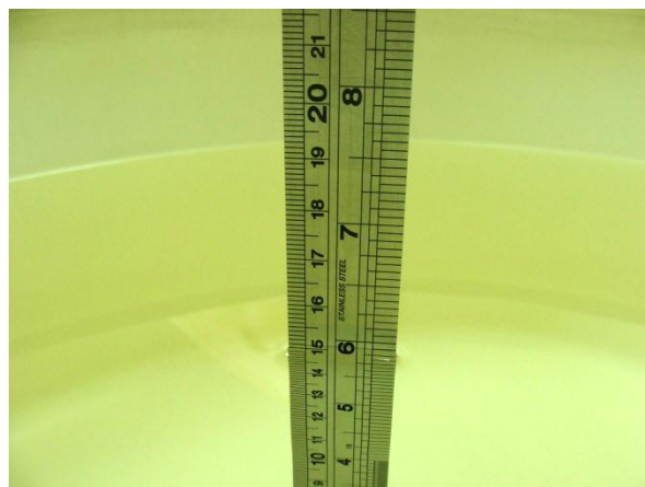
Fig 6.2 Photo of Liquid Height for Body SAR
