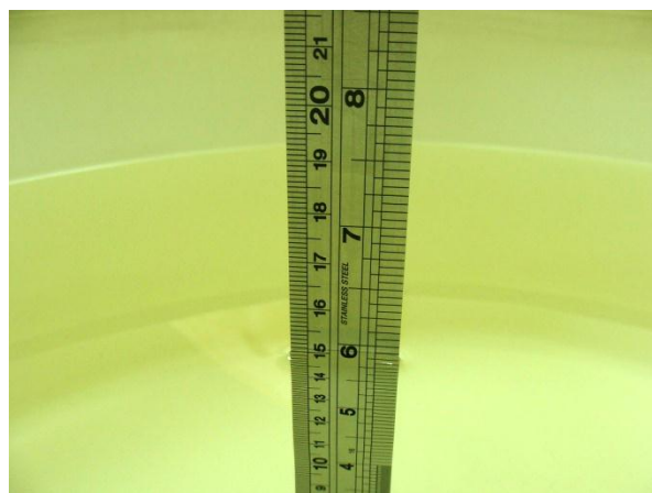
Fig 6.2 Photo of Liquid Height for Body SAR
