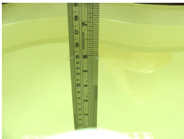
Fig 6.1 Photo of Liquid Height for Head SAR
