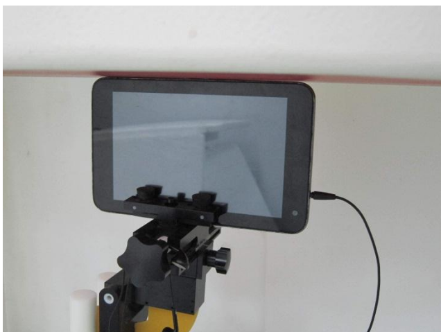
Primary Landscape with Phantom 0 cm Gap for Earphone
