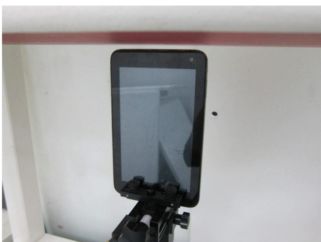
Secondary Portrait with Phantom 0.4 cm Gap for Earphone
