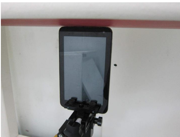
Secondary Portrait with Phantom 0 cm Gap for Earphone
