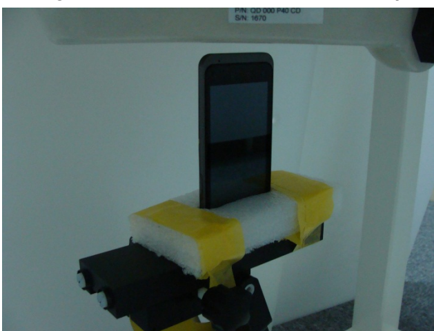
Bottom Side of DUT with Phantom 1 cm Gap
