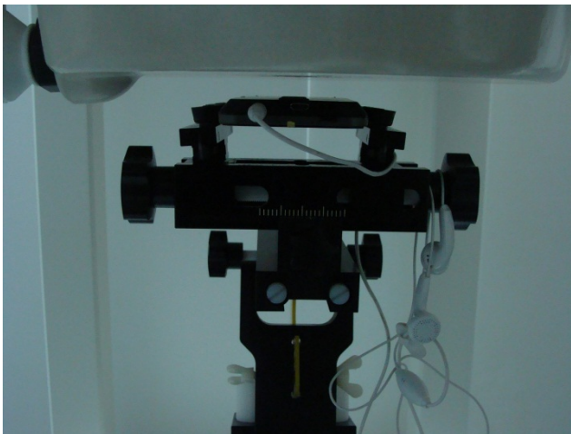
Back of DUT with Earphone to Phantom 1 cm Gap
