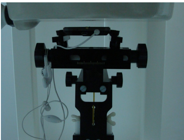
Front of DUT with Earphone to Phantom 1 cm Gap
