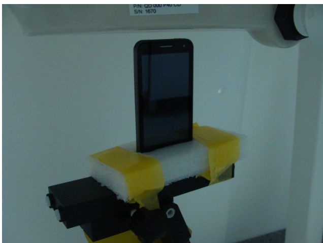
Top Side of DUT with Phantom 1 cm Gap
