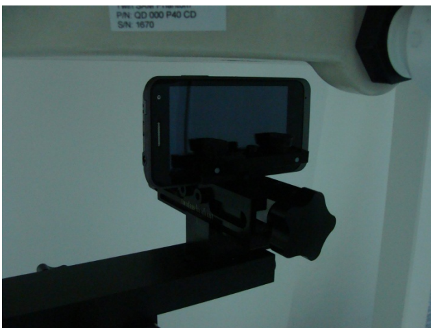
Right Side of DUT with Phantom 1 cm Gap
