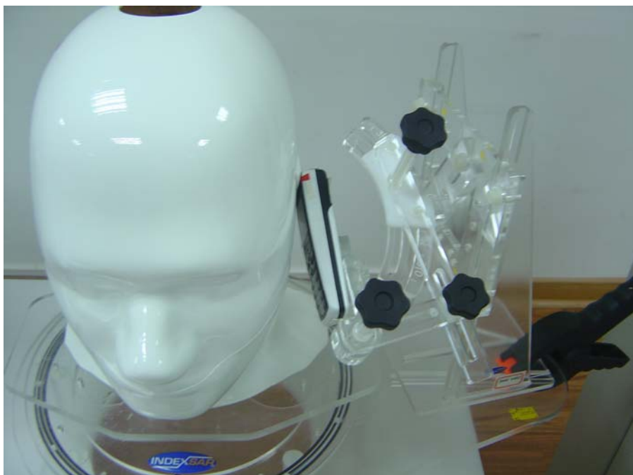
Fig.4 EUT Left Head Tilt15 Position
