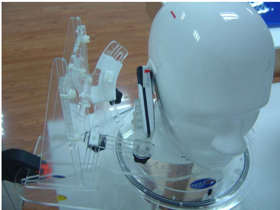
Fig.6 EUT Right Head Tilt15 Position
