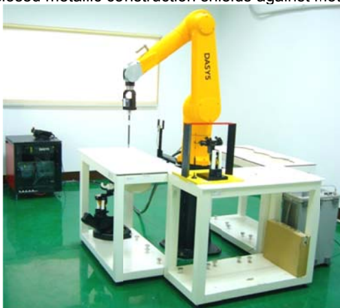
Fig 5.5 Photo of DASY5
