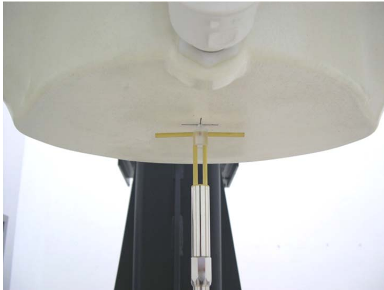
Fig 8.2 Photo of Dipole Setup
