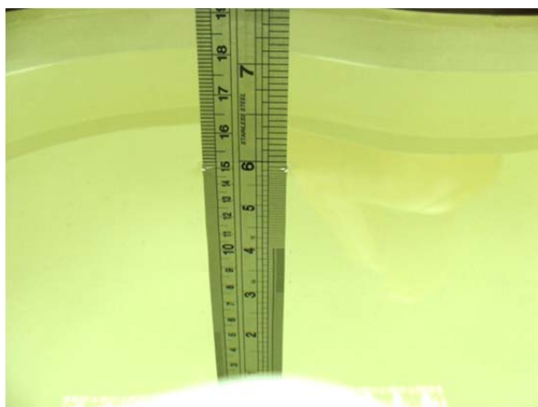
Fig 6.1 Photo of Liquid Height for Head SAR
