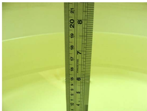
Fig 6.2 Photo of Liquid Height for Body SAR
