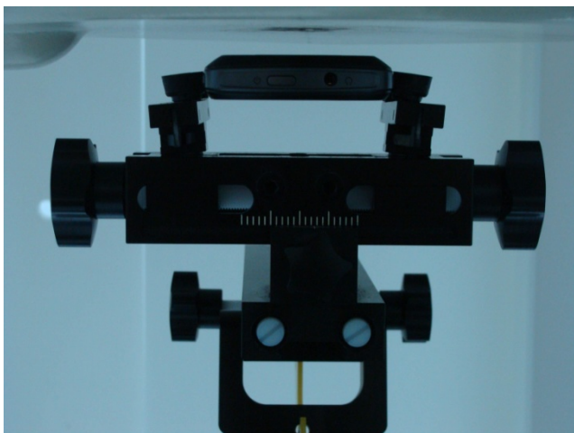
Back of DUT with Phantom 1 cm Gap
