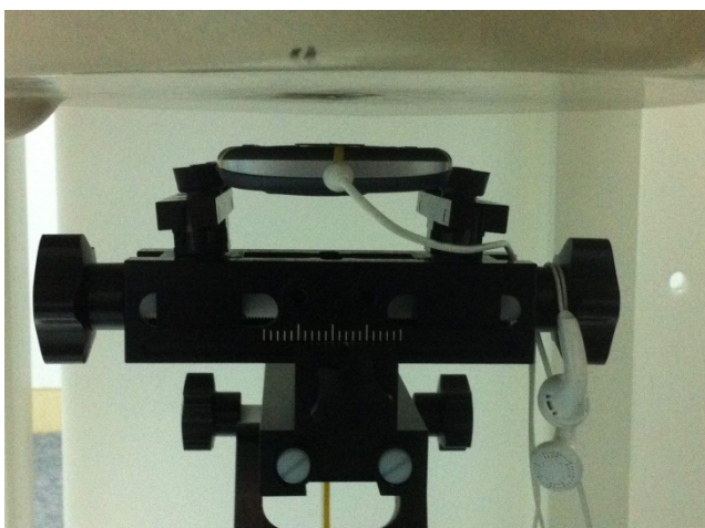
Front of the DUT with Phantom 1.5 cm Gap (Headset)
