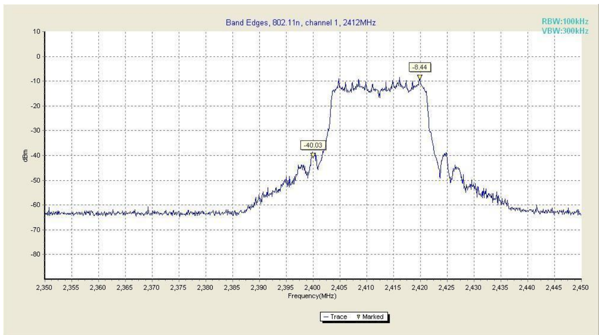
Fig. 23 Band Edges (802.11 n-20MHz, Ch 1)
