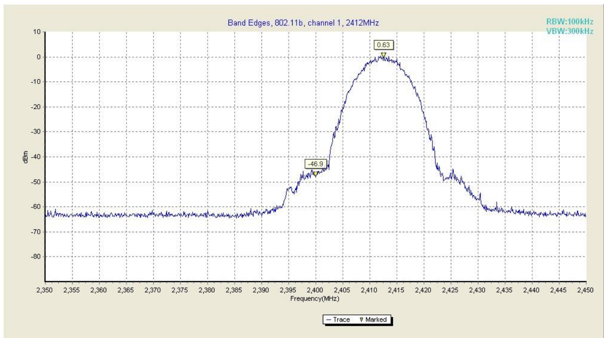
Fig. 19 Band Edges (802.11b, Ch 1)
