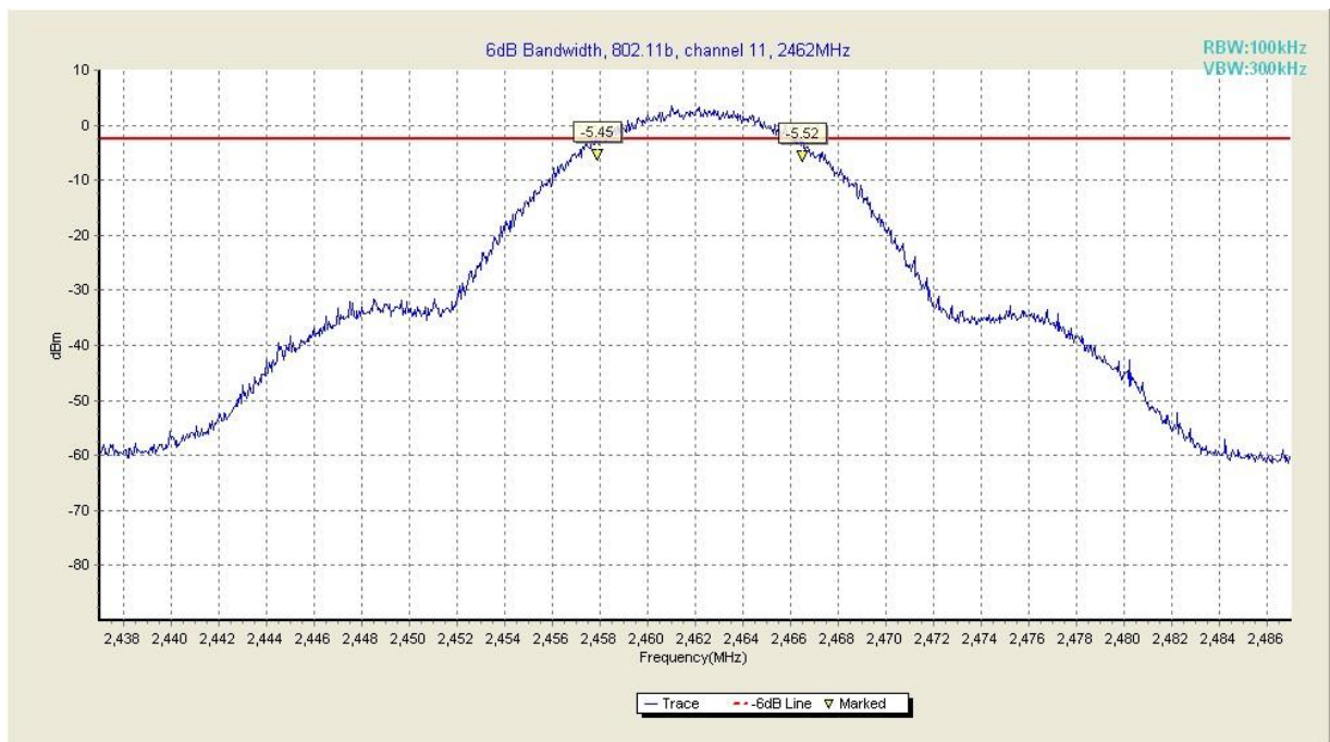
Fig. 12 Occupied 6dB Bandwidth (802.11b, Ch 11)
