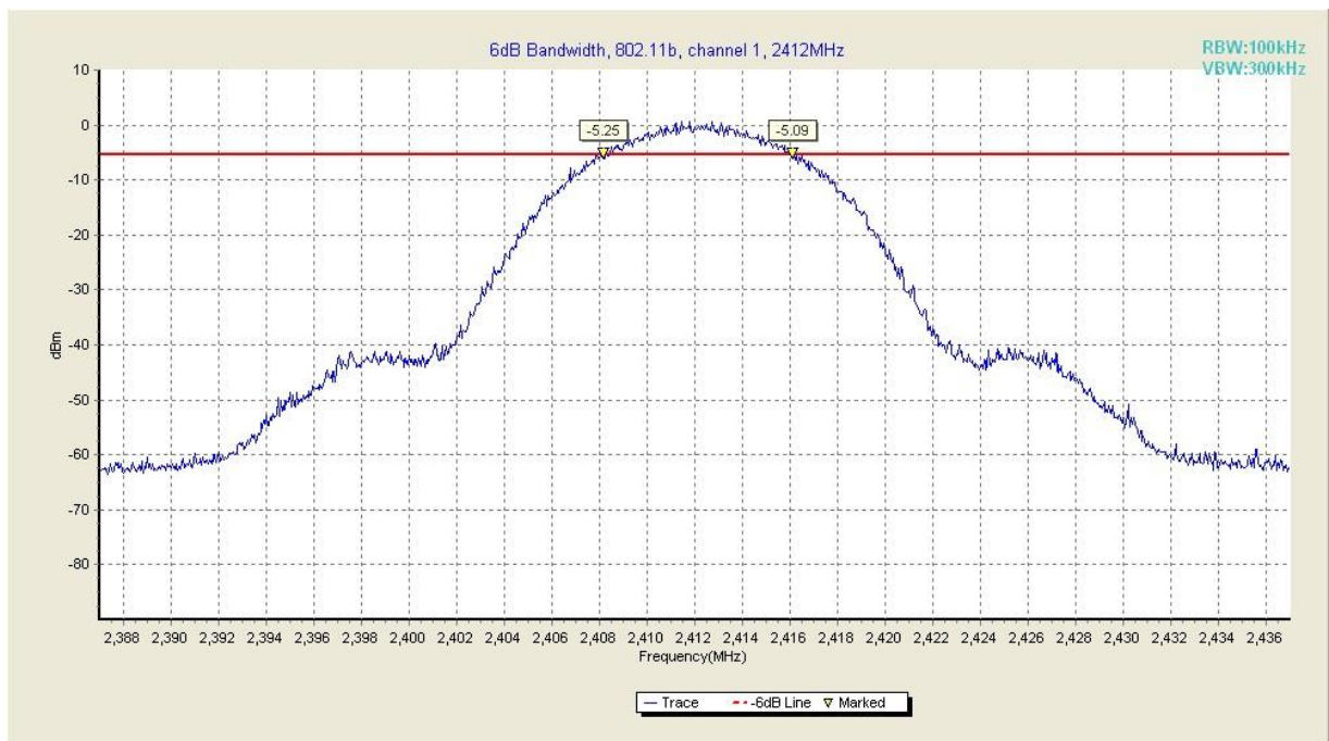
Fig. 10 Occupied 6dB Bandwidth (802.11b, Ch 1)
