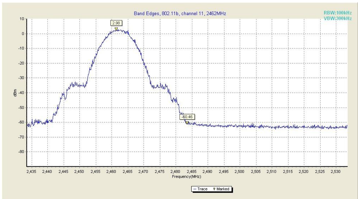
Fig. 20 Band Edges (802.11b, Ch 11)
