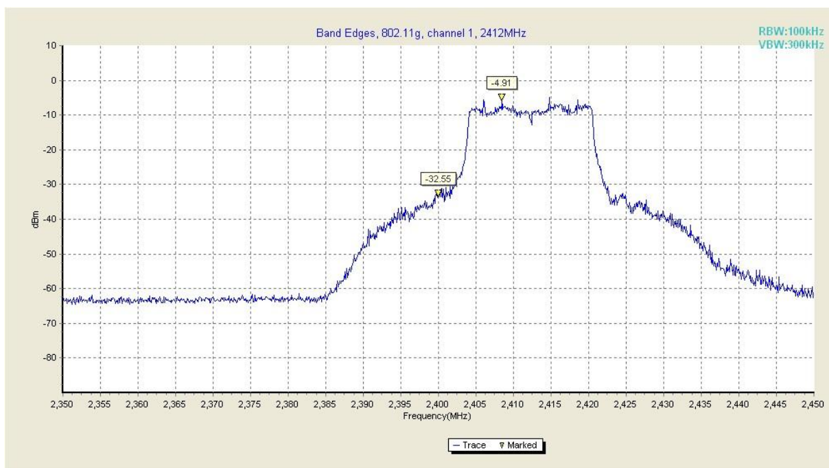
Fig. 21 Band Edges (802.11g, Ch 1)
