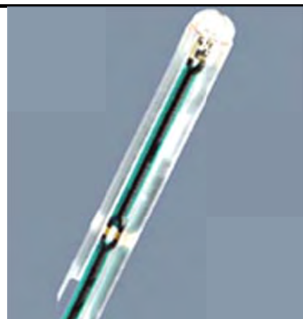
Fig 5.3 Photo of H-field Probe
