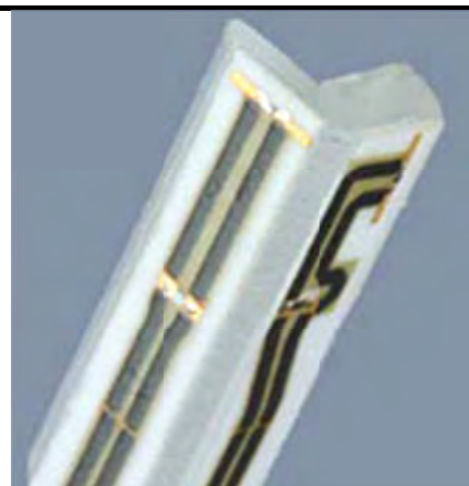
Fig 5.2 Photo of E-field Probe
