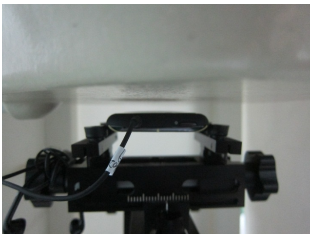
Back of the DUT with Phantom 1 cm Gap (Headset)
