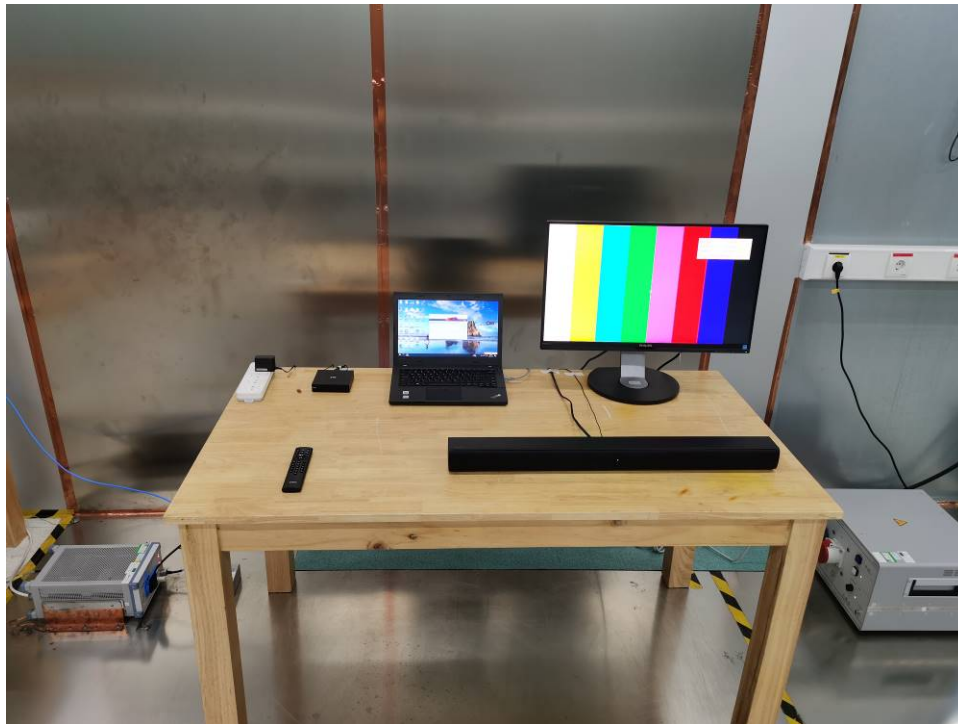
Photograph 3: Set-up for Conducted Emission on AC Mains
