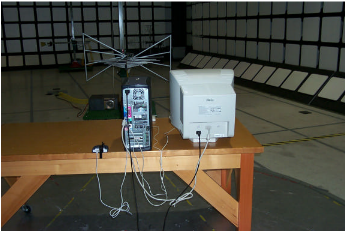
Figure 2 - Radiated Emissions Test Setup
