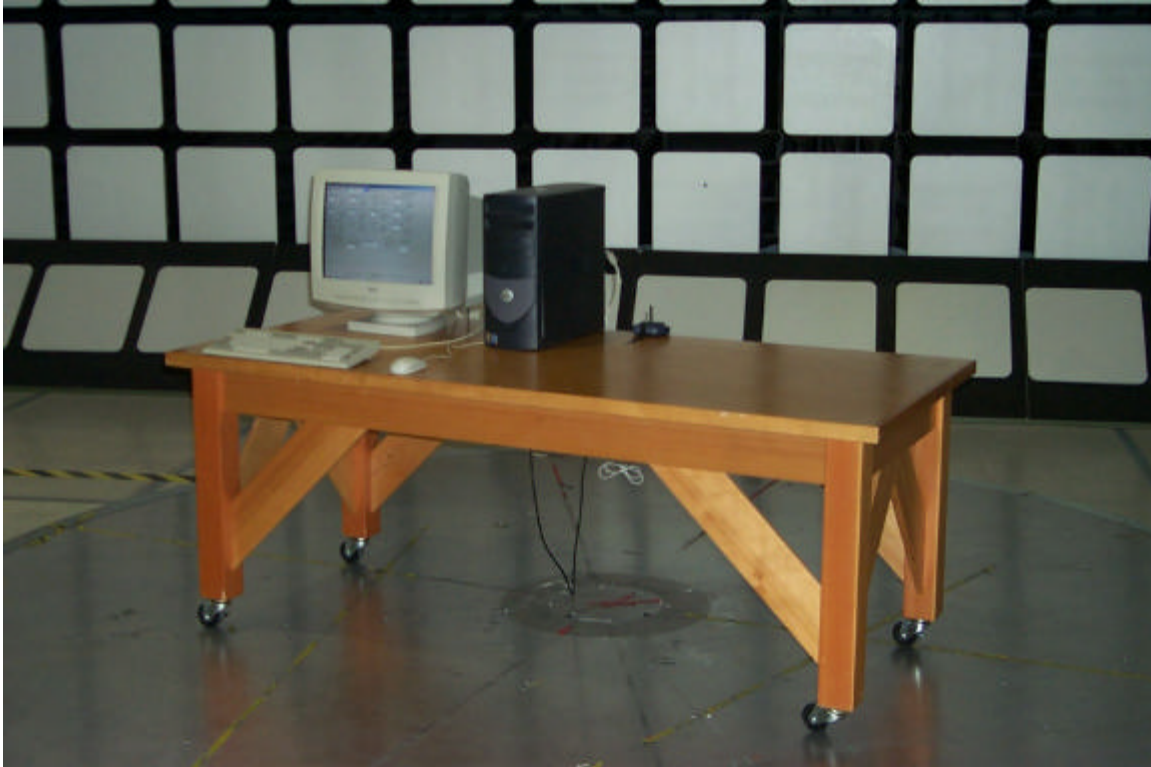
Figure 1 - Radiated Emissions Test Setup
