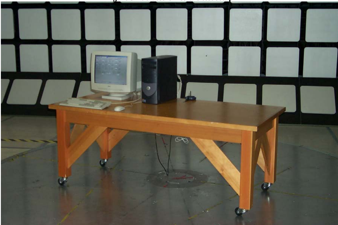
Figure 4 Radiated emissions test setup
