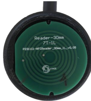
Figure 2 - Antenna Internal Photo - PCB Trace - Bottom View
