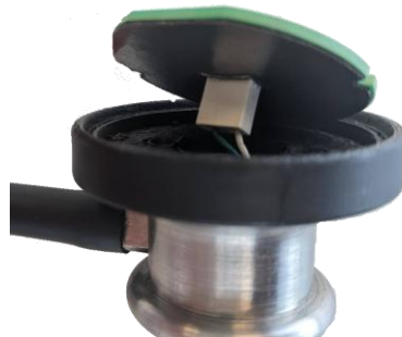
Figure 3 - Antenna Internal Photo – Connector Side
