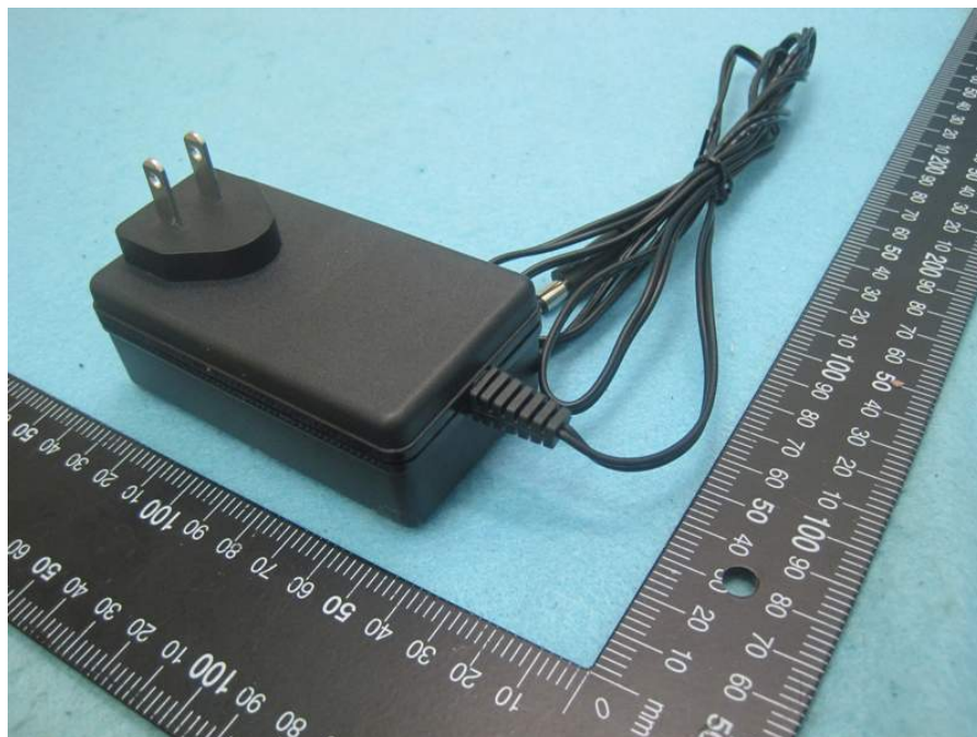
Adapter 3 (Fixed plug) Model No.: HK-X142-12A
