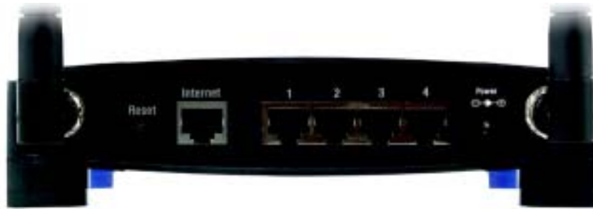
Figure 3-1: The Broadband Router's Back Panel
