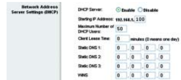
Figure 6-10: Network Address Server Settings
