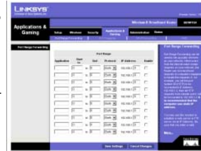
Figure 5-24: Applications and Gaming Tab - Port Range Forwarding
