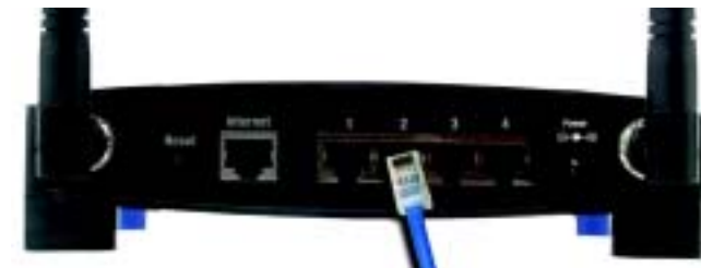
Figure 4-2: Connecting Your Network Devices
