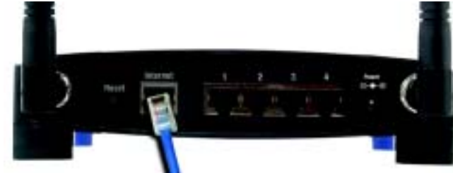
Figure 4-1: Connecting Your Internet Connection
