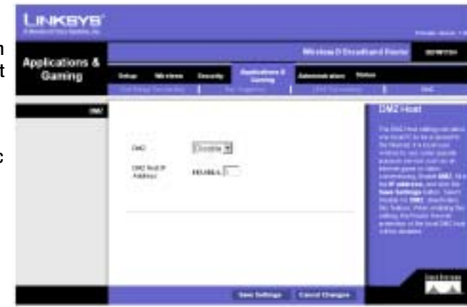
Figure 5-27: Applications and Gaming - DMZ
