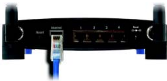
Figure 4-6: Connecting Another Router
