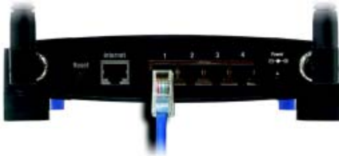
Figure 4-3: Connecting Your Network Devices
