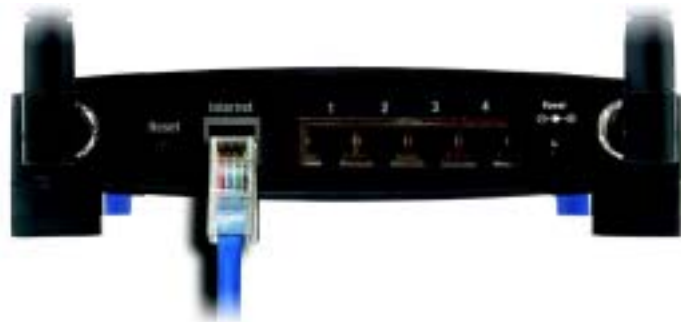
Figure 4-2: Connecting Your Internet Connection
