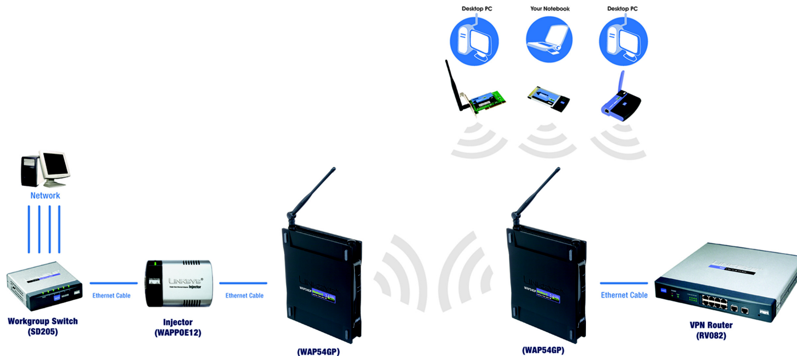
Figure 6-13: Wireless Repeater Diagram
