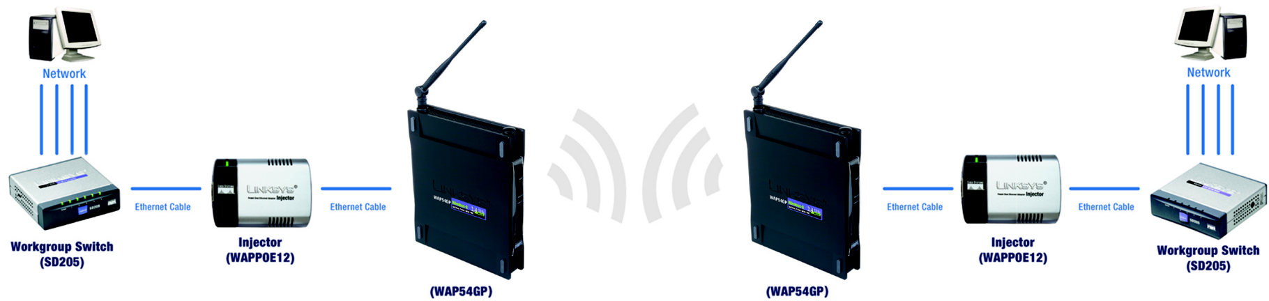
Figure 6-15: Wireless Bridge Diagram
