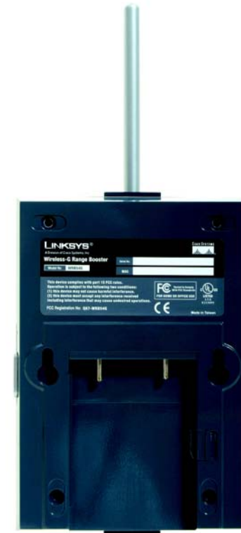
Figure 3-2: Recess for the Power Plate
