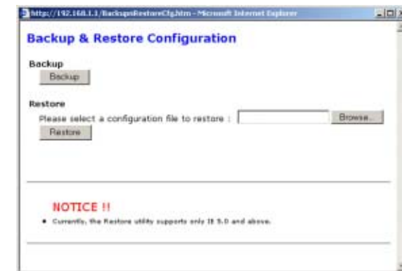
Figure 5-33: Backup and Restore Configuration
