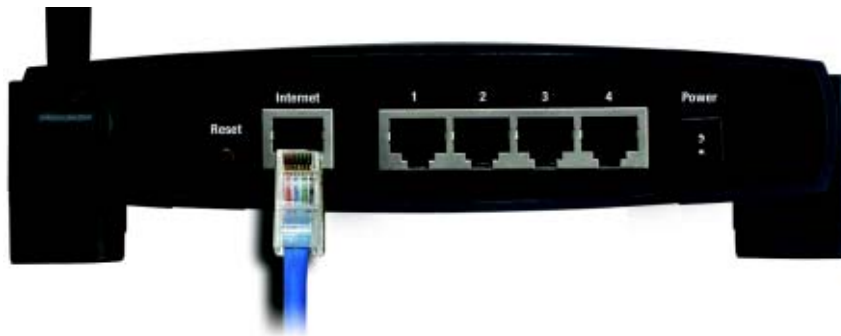
Figure 4-1: Connecting Your Internet Connection
