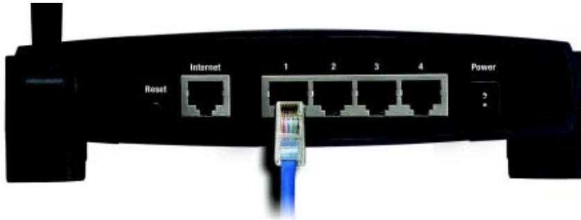
Figure 4-2: Connecting Your Network Devices
