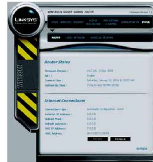
Figure 5-38: STATUS Tab - ROUTER
