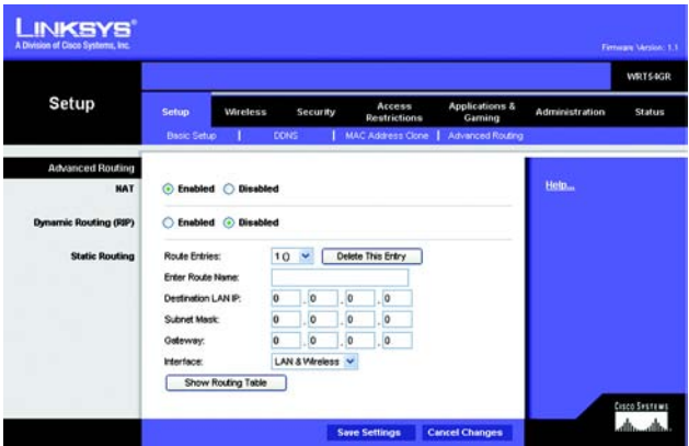
Figure 5-17: Setup Tab - Advanced Routing
